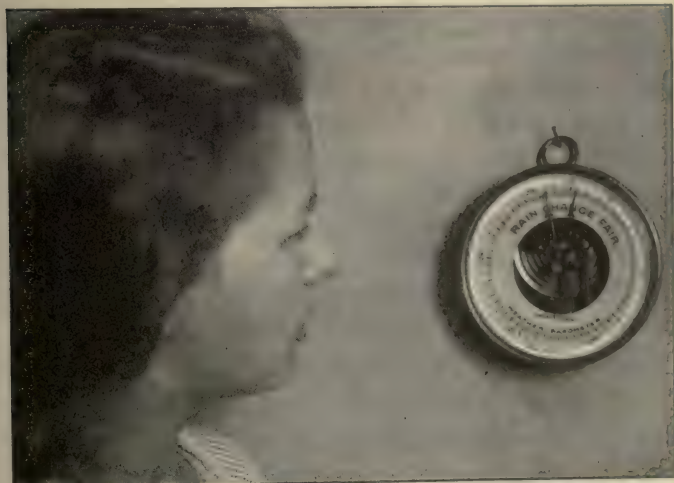
FIG. 156. An aneroid barometer is more convenient than one made with mercury. The walls are forced in or spring back out according to the pressure of the air. This movement of the walls forces the hand around.
